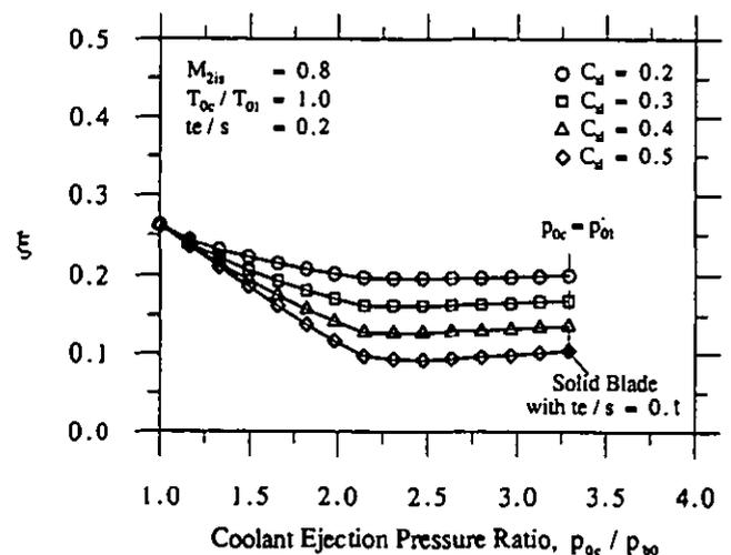
Fig. 3: Variation of Kinetic Energy Loss Coefficient with Coolant Flow
