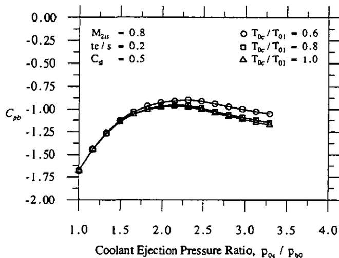
Fig. 4: Influence of Coolant Stagnation Temperature Ratio on Base Pressure Coefficient
