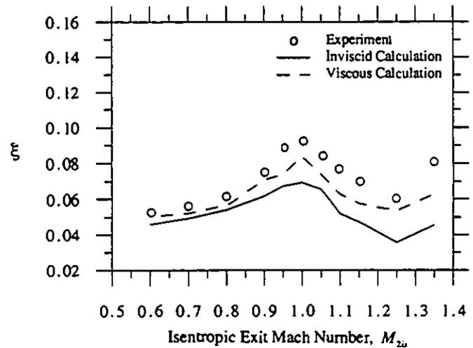
Fig. 12: Predicted and Measured Variation of Loss Coefficient
