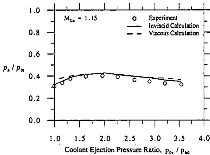
Fig. 16: Predicted and Measured Base Pressures ( $M_{2is} = 1.15$ )
