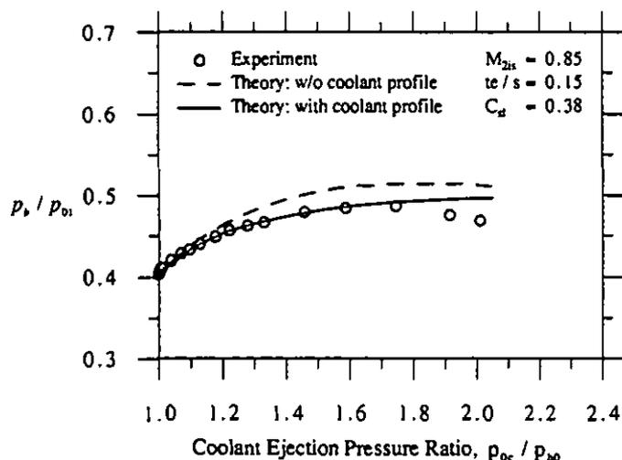
Fig. 6a: Predicted and Measured Base Pressures ( $M_{2u} = 0.85$ )
