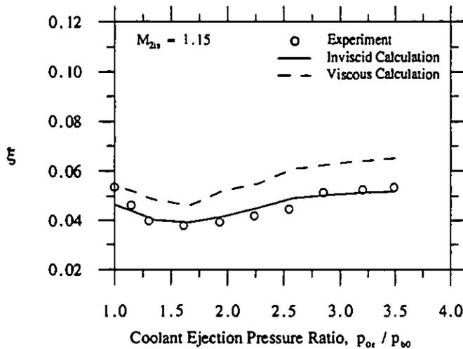
Fig. 17: Predicted and Measured Loss Coefficient ( $M_{2is} = 1.15$ )
