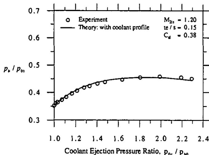
Fig. 6b: Predicted and Measured Base Pressures ( $M_{2u} = 1.20$ )
